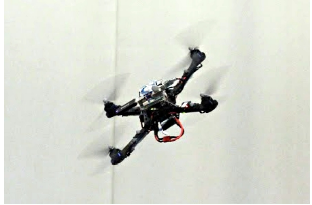
Fig. 1: The Ascending Technologies Hummingbird used in our experiments.
